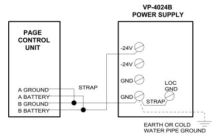
Alternate Ground Method: If using earth or cold water pipe ground, do not connect to LOC GND.
