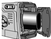
[ Inserting the CR-V3 type battery ]
