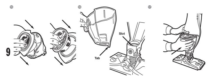
Return the filter to the filter protector and return to the dust canister.
