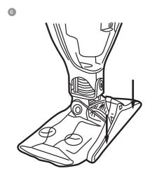
Lift the vacuum nozzle. It should lock into position.
