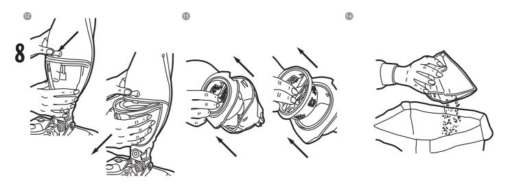
Press the dust canister release button located above the cup on the body of the unit. Tip the dust canister out to remove. Grasp the centre tab on the filter and pull it out of the dust canister. Pull the filter away from the protector. Remove debris from the filter and filter protector. Empty the contents into a waste bin. For best results, shake and lightly tap the filter against the waste bin to remove remaining dirt.
