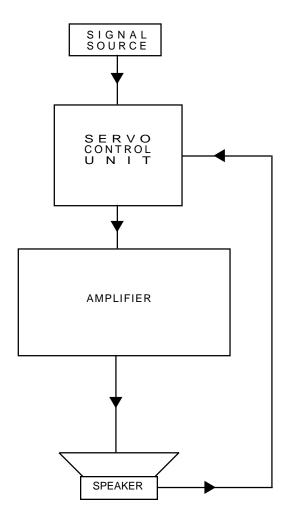
As you can see from this diagram, the speaker and amplifier now become part of a loop. Actual cone motion is monitored, so now we can control the drive signal to the amplifier. In essence, controlling how the speaker responds.
