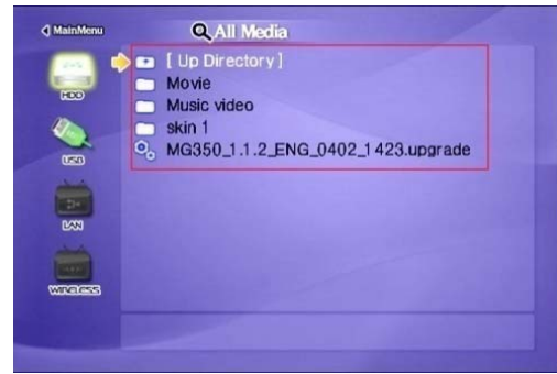
② Data of built-in HDD is displayed. In order to play, select a file and press [OK].
