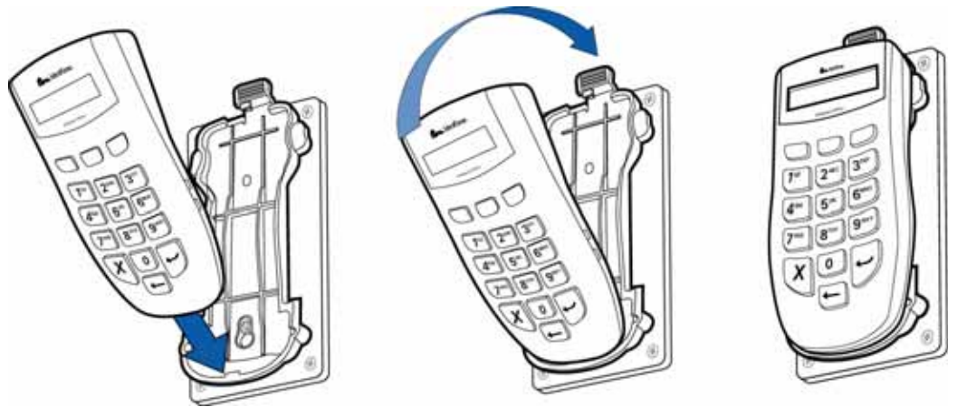
Figure 6 Inserting the PINpad 1000SE device into the Stand Adapter
