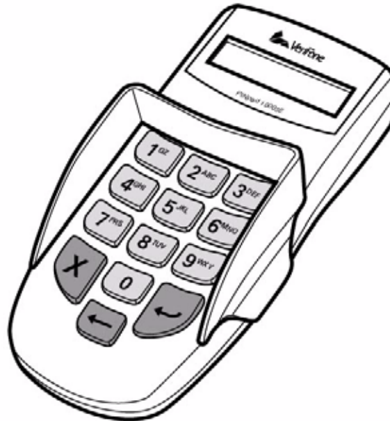
Figure 7 Installed Privacy Shield
