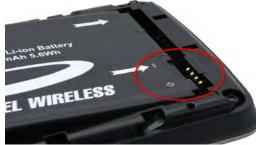
3 Replace the cover by setting it on the device where the notches align, and then gently slide the cover back toward the release button until it clicks into place.
