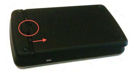
2 Align the gold-colored contacts on the battery with the gold-colored contacts on the device and gently slide the battery into place.
