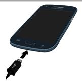
Plug the flat end of the Travel Charger into the charging/USB port and the other end into a standard AC wall outlet. 2. When charging is finished, remove the flat end from the interface connector port on the phone.
