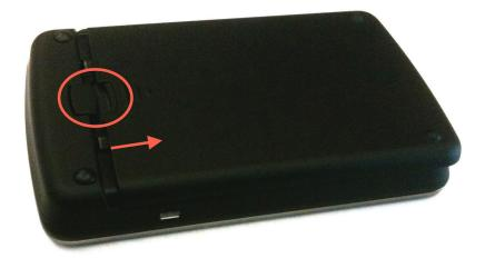
2 Align the gold-colored contacts on the battery with the gold-colored contacts on the device and gently slide the battery into place.
