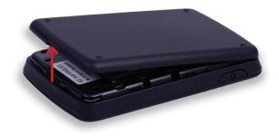
Insert your fingernail into the battery removal divot and lift the battery out of the battery compartment.
