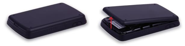
Align the gold-colored contacts on the battery with the gold-colored contacts on the device and gently slide the battery into place.
