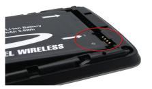
8 Replace the cover by setting it on the device where the notches align, and then press on the cover until it clicks into place.
