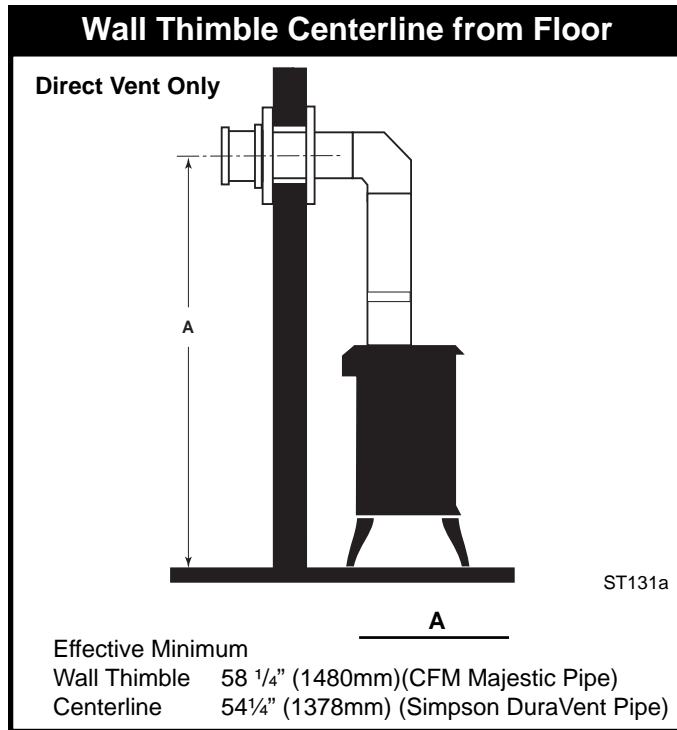
Fig. 5 Minimum wall thimble centerline.
