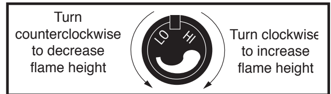
Fig. 47 Flame adjustment knob for Honeywell valve.
