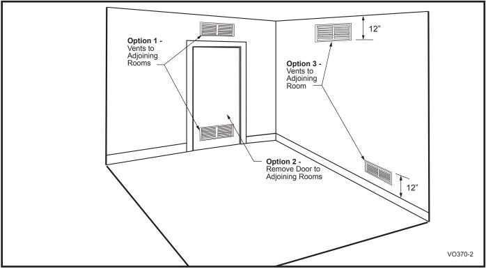
Fig. 2 Ventilaton options for confined spaces.
