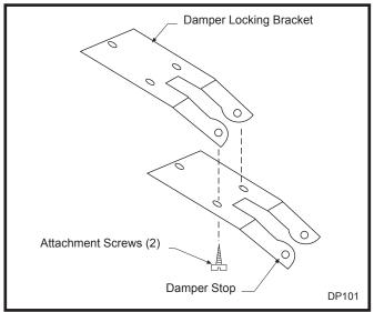
Fig. 5 Attach damper stop.
