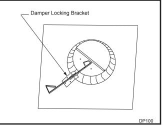
Fig. 4 Locate damper locking bracket.
