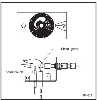
Fig. 15 Correct SIT valve pilot flame.
