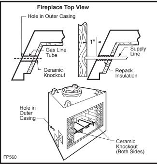
Fig. 3 Gas line installation - factory-built fireplaces.
