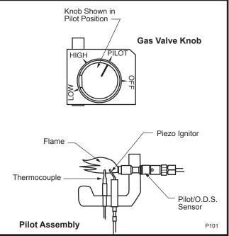
Fig. 14 Typical view of pilot burner flame.
