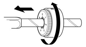
t Slide balanceweight onto rear of tonearm with the number scale facing the cartridge end. Twist lightly to screw into position.
