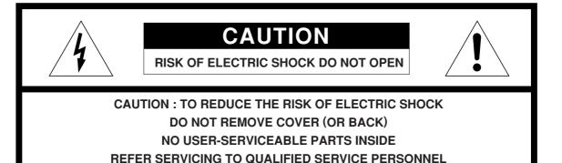
The lightning flash with arrowhead, symbol within an equilateral triangle, is intended to alert the user to the presence of uninsulated "dangerous voltage" within the product's enclosure that may be of sufficient magnitude to constitute a risk of electric shock to persons.
