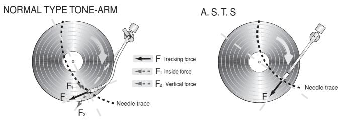
The tracking force (frictional force) generated between the stylus and the record disc makes the inside force. The inside force is minimized.
