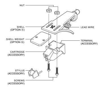
③ The overhang of your cartridge needs to be adjusted to best suit the A.S.T.S tone arm. For best tracking and stylus pressure a distance of 50mm (as shown) should be set.
