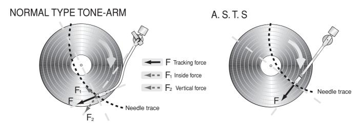
The tracking force (frictional force) generated between the stylus and the record disc makes the inside force.
