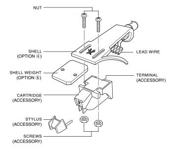
(3) The overhang of your cartridge needs to be adjusted to best suit the A.S.T.S tone arm. For best tracking and stylus pressure a distance of 50mm (as shown) should be set.
