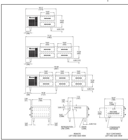
**NOTE:** If cabinet is located directly against wall and/or under low ceiling, a minimum clearance of 2" is required.
