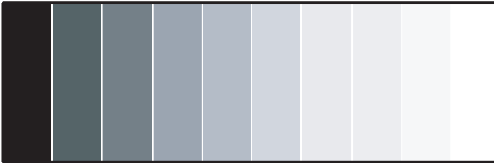
Figure 4-4. Typical Gray Bar Pattern for Adjusting Contrast
