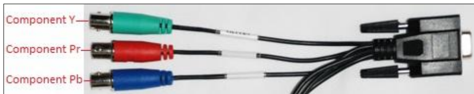
Figure 15. YPrPb dongle connections
