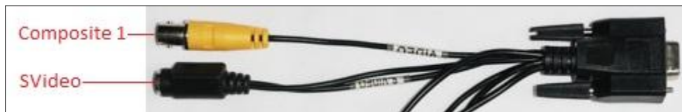
Figure 14. Composite/SVideo dongle connections
