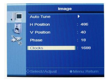
b. Press " " or " " to adjust the clock of signal. Then press "1" to confirm the adjustment and back to Image menu.
