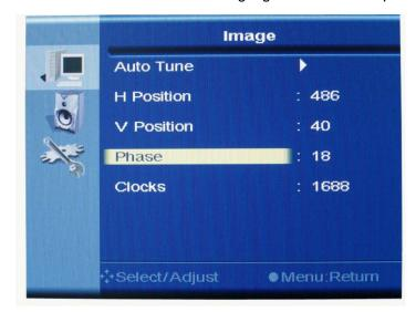
b. Press " " or " " to adjust the phase of signal. Then press "1" to confirm the adjustment and back to Image menu.
