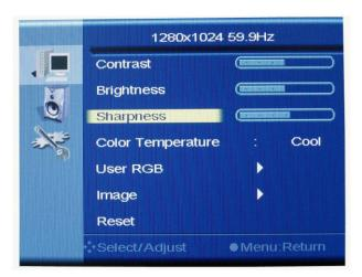
b. Press " " or " " to increase or decrease the sharpness of the display. Press "1" to confirm the adjustment and back to OSD main menu.
