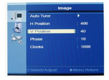
b. Press " " or " " to move the vertical position of OSD . Then press "1" to confirm the adjustment and back to Image menu.
