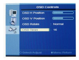
b. Press "1" to adjust the length of time in seconds for which OSD menu appears on the screen. Then press "2" to confirm the adjustment and back to Feature Controls menu.
