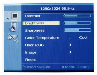
b. Press " " or " " to increase or decrease the brightness of the display. Press "1" to confirm the adjustment and back to OSD main menu.
