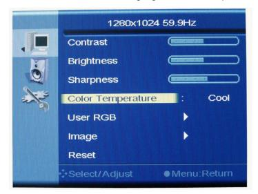
b. Press "1" to select preset color temperature settings, like Cool, Natural, Warm, or select User to adjust Red, Green, Blue independently. If Cool, Natural, or Warm is selected, then press "2" to confirm the selection and press "2" to exit.
