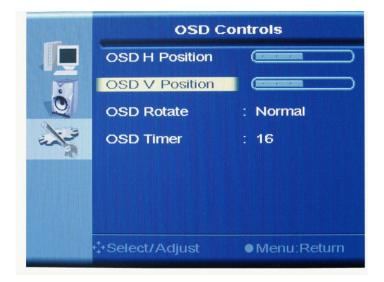
b. Press " " or " " to adjust the vertical position of OSD menu. Then press "1" to confirm the adjustment and back to OSD Control sub-menu.
