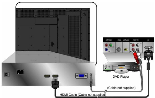
Note: To receive the sound from DVD, please turn on Sound Menu of OSD for selecting HDMI audio to HDMI. However, the input source should be in HDMI.
