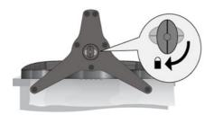
3. Lock up the switch under the base.
