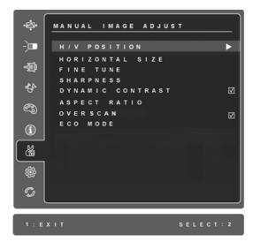
**H./V. Position (Horizontal/Vertical Position)** moves the screen image left or right and up or down.
