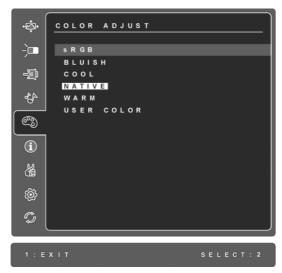
**sRGB-**This is quickly becoming the industry standard for color management, with support being included in many of the latest applications. Enabling this setting allows the LCD display to more accurately display colors the way they were originally intended. Enabling the sRGB setting will cause the Contrast and Brightness adjustments to be disabled.
