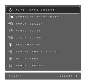
**NOTE:** All OSD menus and adjustment screens disappear automatically after about 15 seconds. This is adjustable through the OSD timeout setting in the setup menu.
