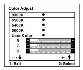
9300K - Adds blue to the screen image for cooler white (used in most office settings with fluorescent lighting).
