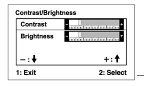
The command line at the bottom of the control screen tells what to do next from this screen. You can toggle between control screens, adjust the selected option, or exit the screen.
