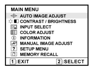
**NOTE:** All OnView menus and adjustment screens disappear automatically after about 15 seconds. This is adjustable through the OSD timeout setting in the setup menu.
