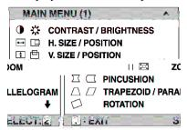
2 To select a control you want to adjust, press the arrow buttons on the front control panel of your monitor and scroll through the choices. When the control you want is highlighted, press button [2].
