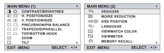
2. To select a setting to be adjusted, press the arrow buttons on the front control panel of your monitor and scroll through the choices. When the desired control is highlighted, press button ◀/▶.
