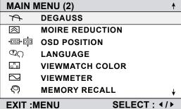
2. To select a setting to be adjusted, press the arrow buttons on the front control panel of your monitor and scroll through the choices. When the desired control is highlighted, press button ◀/▶.
