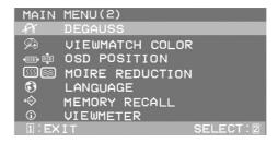
2 To select a control you want to adjust, press the arrow buttons on the front control panel of your monitor and scroll through the choices. When the control you want is highlighted, press button [2].
