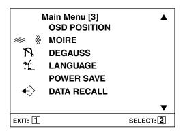
**OSD POSITION** allows you to reposition the OnView display (including all menus and control screens). Press  $[\nabla]$  or  $[\Delta]$  to move the OSD. To exit this screen, press button [1].
