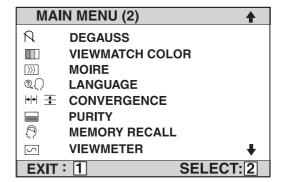
2 To select a control you want to adjust, press the arrow buttons on the front control panel of your monitor and scroll through the choices. When the control you want is highlighted, press button [2].
