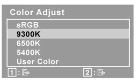
**sRGB-**This is quickly becoming the industry standard for color management, with support being included in many of the latest applications. Enabling this setting allows the LCD display to more accurately display colors the way they were originally intended. Enabling the sRGB setting will cause the Contrast and Brightness adjustments to be disabled.
