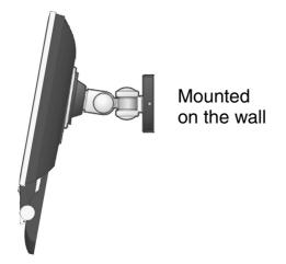
**5** Attach the LCD display to the wall, following the instructions in the wall-mounting kit.
