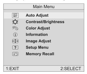
**NOTE:** All OnView menus and adjustment screens disappear automatically after about 15 seconds. This time period is adjustable through the Setup menu and the OSD timeout control described on page 11.
