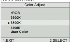
**sRGB** — sRGB is quickly becoming the industry standard for color management, with support being included in many of the latest applications. Enabling this setting allows the LCD display to more accurately display colors the way they were originally intended. Enabling the sRGB setting will cause the Contrast and Brightness adjustments to be disabled.
