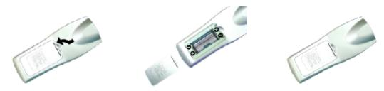
1 Remove the battery cover by pulling then lifting the knob on the cover.
