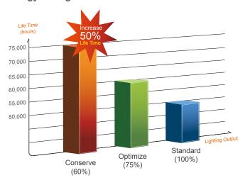
The ECO Mode function comes standard with all LED displays. Select from the "Optimize (75%)" or "Conserve (60%)" options to reduce display brightness and save up to 40% energy. Especially under low ambient light conditions, adjusting the brightness will improve visibility by reducing eye fatigue. It will also prolong the display's lamp life, helping you save money and save the planet.
