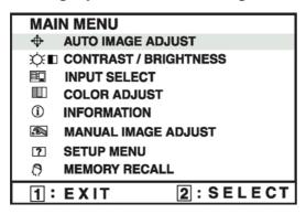
**NOTE:** All OnView menus and adjustment screens disappear automatically after about 15 seconds. This is adjustable through the OSD timeout setting in the setup menu.
