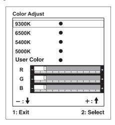
**9300K** — Adds blue to the screen image for cooler white (used in most office settings with fluorescent lighting).
