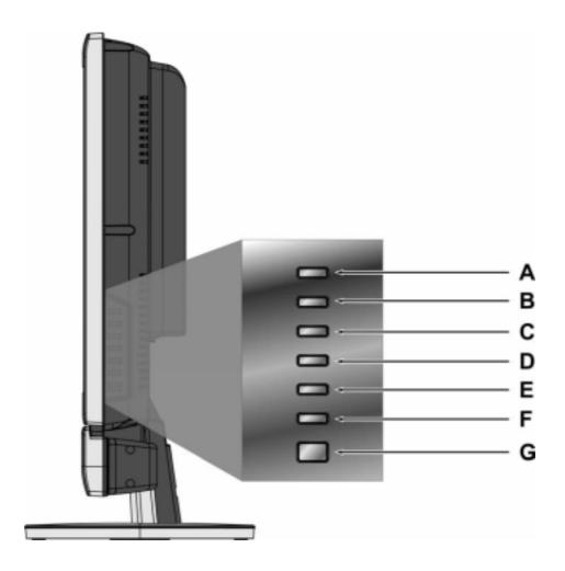
Α Input Select the Input source. Confirm OSD menu selection. В **Volume Up** Increase volume or adjust a highlighted increasingly control while in OSD menu. C **Volume Down** Decrease volume or adjust a highlighted control decreasingly while in OSD menu. CH Up D Channel up/ Scroll up. Ε **CH Down** Channel down/ Scroll down. F Turn OSD menu ON/OFF. Power G
