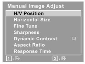
**H./V. Position (Horizontal/Vertical Position)** moves the screen image left or right and up or down.
