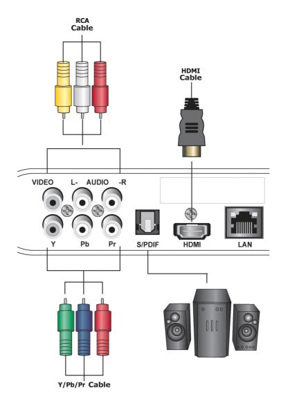
Plug the Ethernet cable to the "LAN" jack on the rear panel of VMP72, for wired Internet connection. VMP72 will detect the network automatically.
