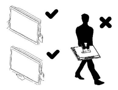
[Attention] Hold firmly when carry the computer, do not grasp the support frame directly.
