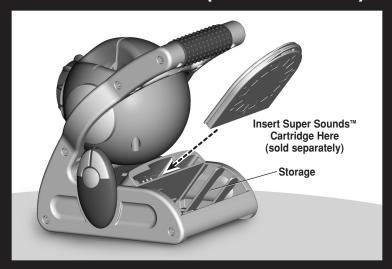
9. Insert the matching Super Sounds™ 3D audio cartridge into the upper slot under the handle.
