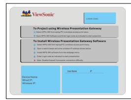
If you can see this start screen display on projector, indicates WPG-360 is working and all connection cables are correctly connected.
