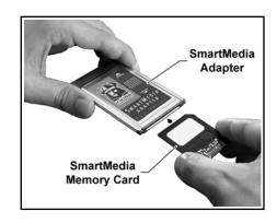
2. Insert the adapter with the Viking logo on its label facing up into one of your computer's PC Card slot. Then firmly press the card into the slot to ensure it is completely seat-
