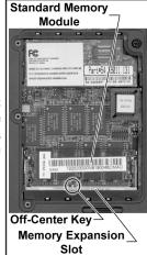
5. In order to upgrade your system past 32MB of memory, its standard memory module will need to be removed. To remove a memory module, locate the retaining clips on both sides of the memory module. Gently pull both clips away from the module and then lift the module out of its expansion slot.
