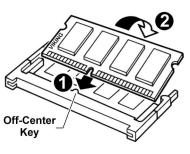
Note: For optimum performance, install the largest capacity memory module into the top expansion slot.
