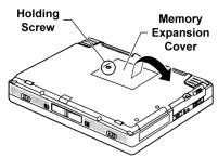
3. Locate the memory expansion cover on the right side of the bottom panel. Also locate its single holding screw. Use a small Phillips screwdriver to remove the holding screw. Then remove the cover by lifting it to the right.
