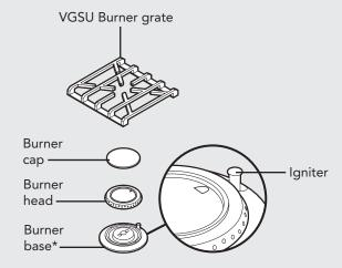
**\*Note:** When replacing burner head, carefully align the tab underneath the cap with the slot in the burner base.
