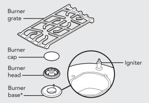
\*Note: When replacing burner head, carefully align the tab underneath the cap with the slot in the burner base.
