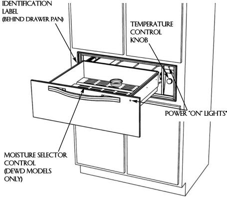
\*The DEWD model has a power "ON" indicator light located on both the control panel and the door front. The DFWD model only has a power "ON" indicator light located on the control panel.
