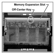
4. Locate the memory expansion slot at the top of the open compartment. Notice the location of the slots off-center key.
